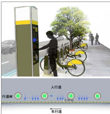
图8 行道树间的立柱式公共自行车租赁点设计指引 Fig.8 Design guidelines for pole-type public bicycle rental stations
