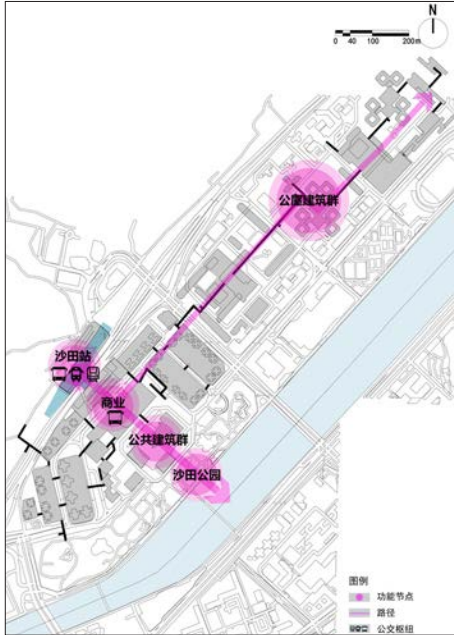
图4 香港沙田空中步行系统空间组织图 Fig.4 Spatial organization of urban elevated walking system in Shatin, Hong Kong
