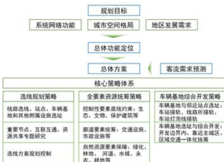
图8 市域铁路选线规划决策路径 Fig.8 Decision path for suburban railway line selection planning
