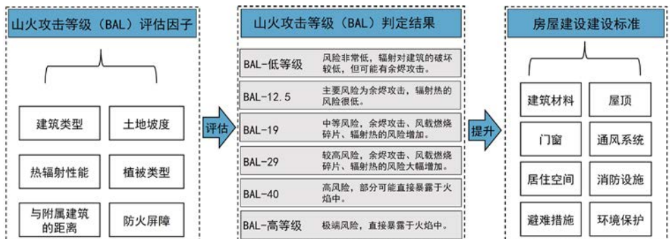
图3 房屋山火攻击等级评估与建设标准改善 Fig.3 Evaluation of house hill fire attack level and improvement of construction standard
