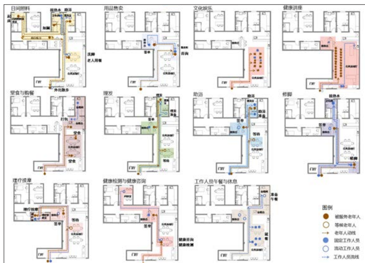
图10 D-2驿站内各服务项目与功能空间对应关系 Fig.10 The corresponding relationship between service options and functional spaces in station D-2
