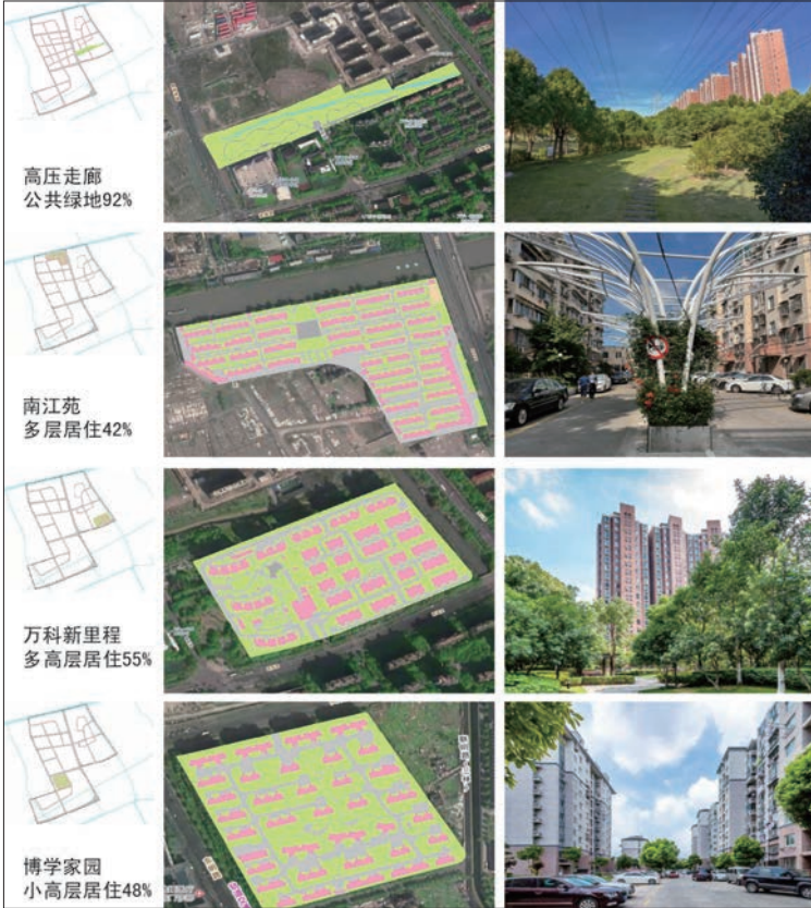
图8 浦东新区杨思地区典型地块海绵城市指标（年径流控制率）评估 Fig.8 Simulation analysis of sponge city indicators of various types of current land use in Yangsi Area, Pudong New Area
