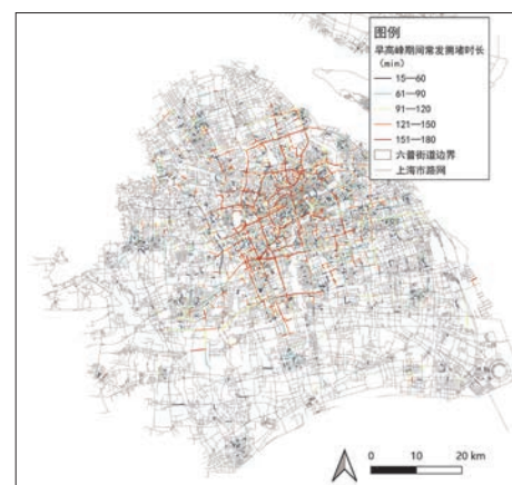
图2 常发拥堵路段的平均拥堵时长 Fig.2 Average duration of congestion on regular congested roads
