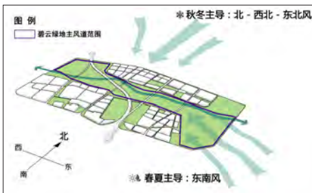
图5 碧云绿地主风道控制分析图 Fig.5 Main air duct control analysis diagram of "Green City Green Park"
