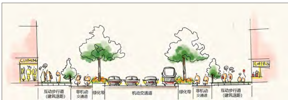
图2 街道宽度及建筑退距示意图 Fig.2 Street width and building setback distance
