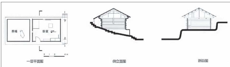
图3 独龙族传统木垒房测绘图纸 Fig.3 Map drawing of a traditional Dulong wooden house
