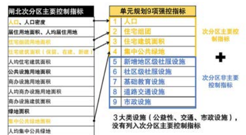
图5 次分区和单元规划控制指标不对应的情况 Fig.5 Control indicators mismatch between sub division and unit planning
