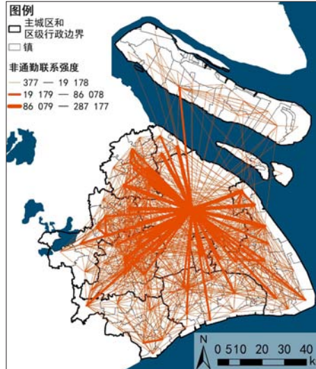
图3 手机信令数据得到的居民跨镇非通勤网络 Fig.3 Network of residents' inter-town non-commuting trips by mobile phone signaling data
